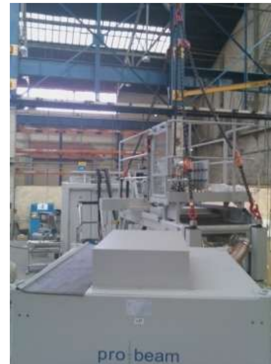
Local vacuum Electro Beam welding machine (CNIM)
