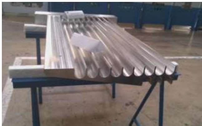
Machined side radial plate segment (CNIM)
