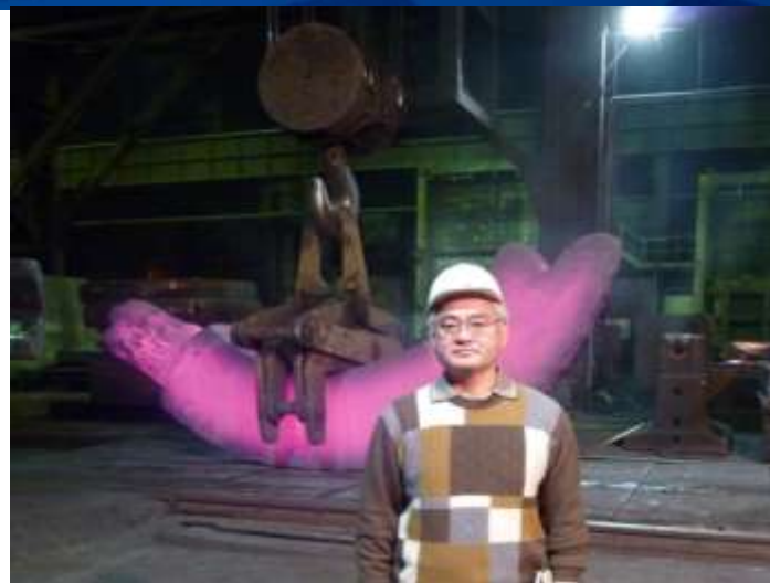
Prototype of side plate for TF coil case under forging process (above) and finished shape (below)
