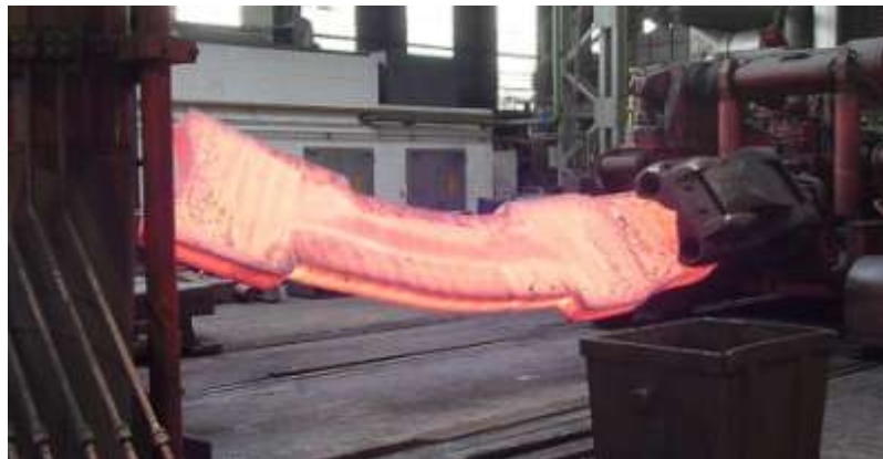
Forging of radial plate segmentt (CNIM)
