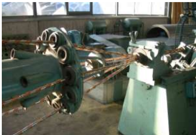
Final stage (5th) cabling around central spiral
