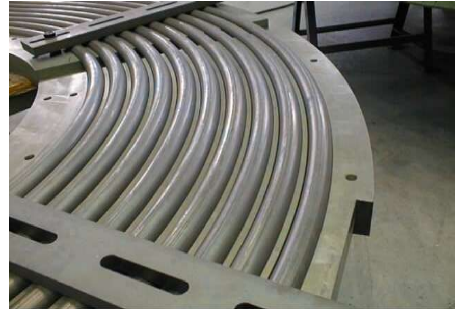
After HT: Gap on INTERNAL side of groove
