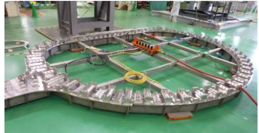
1-3 scale winding table for TF coil prototype (JA)
