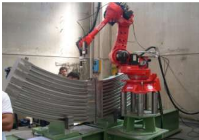
Assembly of radial plate with MAG welding (in progress at SIMIC)
