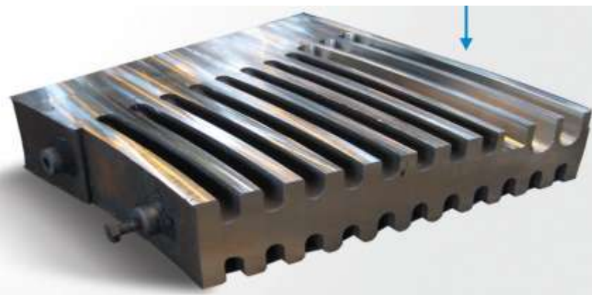
Radial plate segment produced by powder HIPping (SIMIC)
