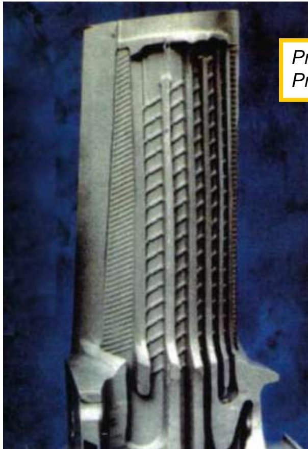
Gasturbine blade cooling
