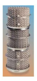
Packed columns for HCLL TEU contain the metal filler Mellapak 750Y. TEU has variable operational temperature up to 450° C.
