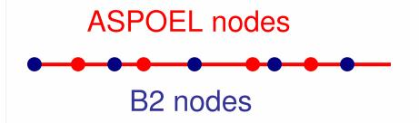
Nodes are not coincident at the interface surface → interpolation is needed
