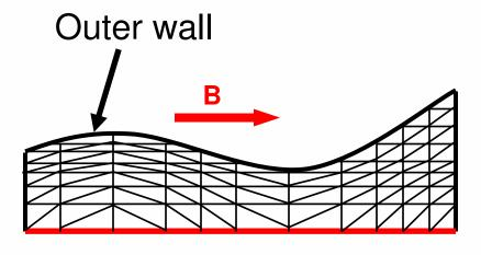
ASPOEL meshes are accurately aligned to B and interpolate the FW geometry
