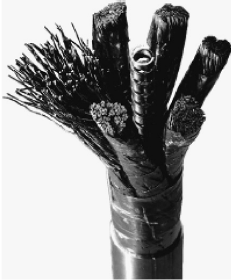
Fig. 1. Build-up of a typical ITER CICC with multi-stage cable inside a circular jacket and around the central channel delimited by a spiral (central channel inner diameter D_{in} = 10 mm and spiral thickness h = 1 mm in this picture).
