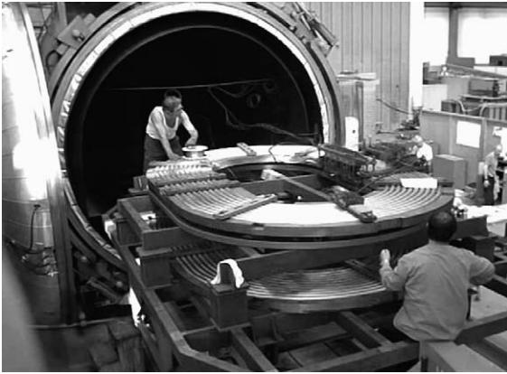
Fig. 3.6. Two pancakes in the reaction moulds in front of the furnace.
