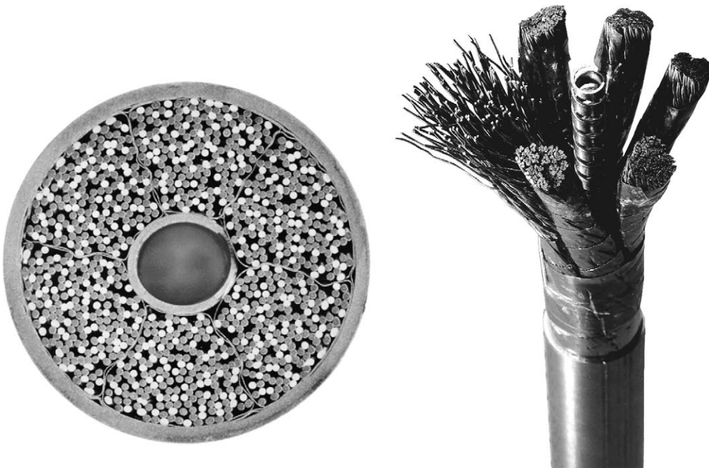
Fig. 3.3. Cross-section and build-up of the TFMC conductor.
