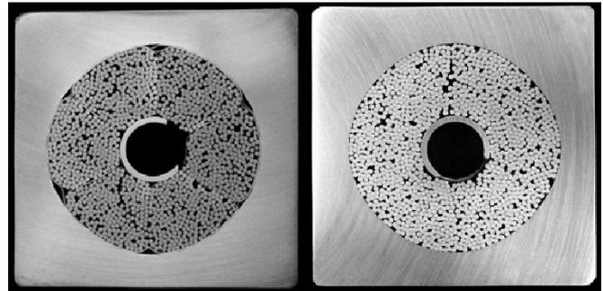
Fig. 1. PFCI NbTi forced flow cable-in-conduit conductors, with wraps (left) and without wraps (right). The two photos have slightly different scale, and the outer size of both conductors is given in the text.
