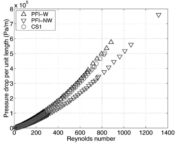
Fig. 5. Pressure drop per unit length as a function of Reynolds number. The results of the ITER CS conductor (with wraps) are also included for comparison with the PFCI conductor with wraps.
