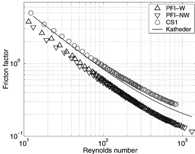
Fig. 6. Comparison of experimental results of the PFCI and CS conductors (open symbols) with the Katheder correlation. For the latter, only the PFI<sub>NW</sub> curve with  $v = 34.31\%$  is shown (see text).
