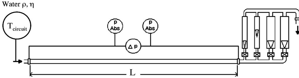
Fig. 2. Schematic view of the experimental set-up, showing the differential and absolute pressure sensors at inlet/outlet, and the floating-ball flow meters. The thermometer is used to derive the average thermodynamic properties of the water. Values of the sample length  $L$  are listed in Table I.
