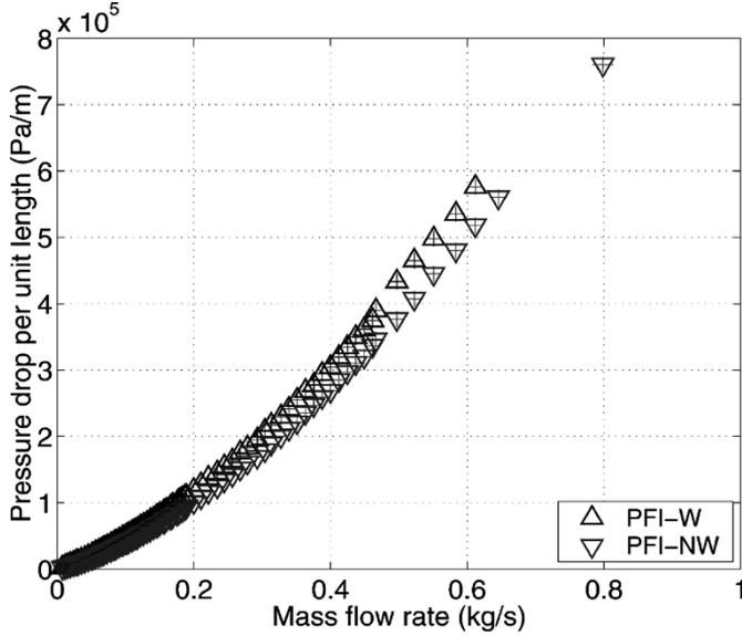
Fig. 3. Results of the raw measurements, including the error bars (inside the symbols).
