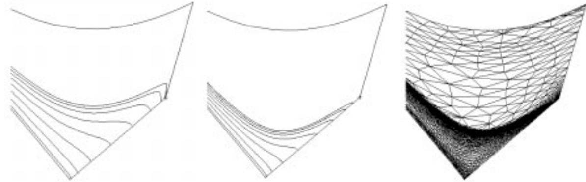
Figure 4 “Detachment” transient simulated by increasing the amplitude S of the nonlinear radiation sink S(u) . Zooms of the computational domain including X-point (lowermost point) region and oblique target on the right. Attached solution for S=1e7 (left) used as initial condition for evolution to detached steady state with S=2e7 (center). Final adaptive mesh with 12631 nodes (right).
