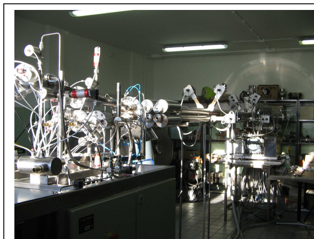
Figure 2. The Ignitor Pellet Injector propelling sub-system built by ENEA at Criotec Impianti.
