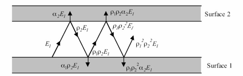
Consider the two infinite gray surfaces shown in Figure . We suppose that the surfaces are thick enough so that,  $\alpha + \rho = 1$  (no radiation transmitted so transmittance = 0). Consider a photon emitted from Surface 1 (remembering that the reflectance  $\rho = 1 - \alpha$ ):
