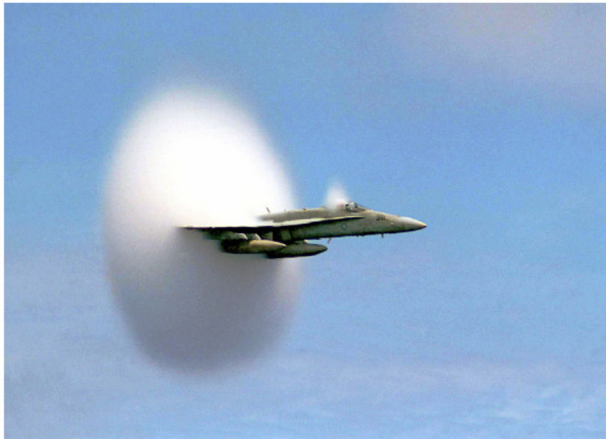
Condensation fronts in the flow around a transonic F/A-18 Hornet operating in humid conditions. U.S. Navy photograph by Ensign John Gay.
