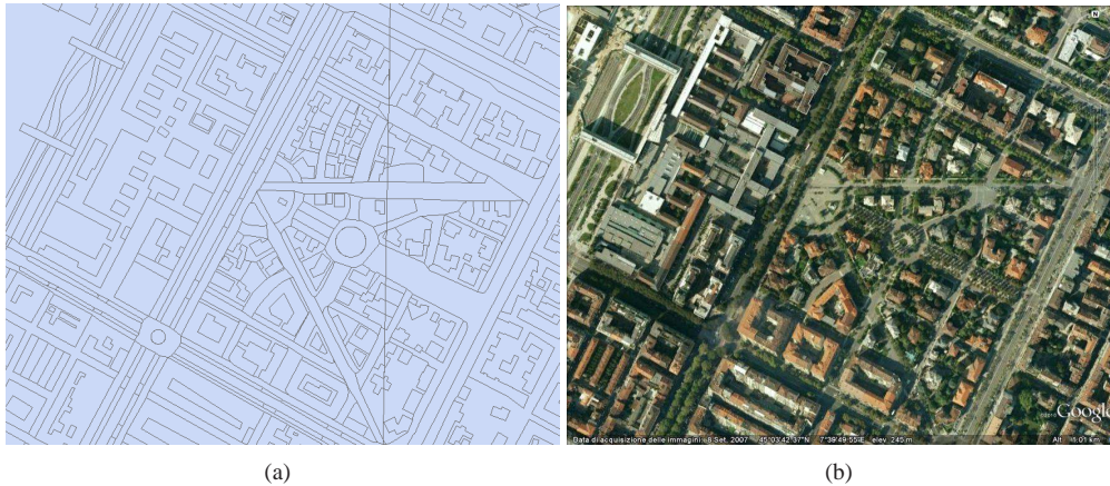
Figure 4: Comparison of the Piedmont numerical map (a) with the Google Earth™ image (b) for the same location. The snapshots show a view of Politecnico di Torino and neighborhood. In the view from the numerical map (a) it is possible to see the edge where two sections have been merged.
