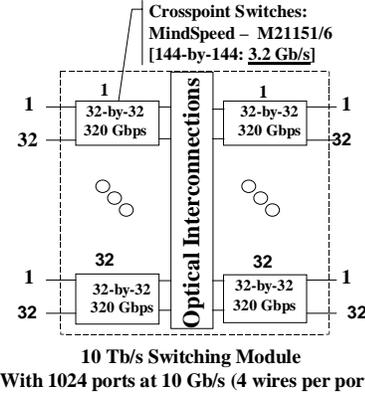
Figure 2. 10 Tb/s Switching with M21151/6 cross-point
