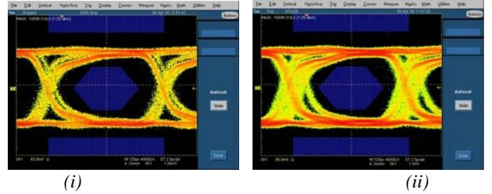
Figure 7: Eye Pattern at (i) location B and (ii) location C
