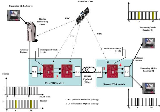
Figure 4: Initial testbed with two TDS nodes
