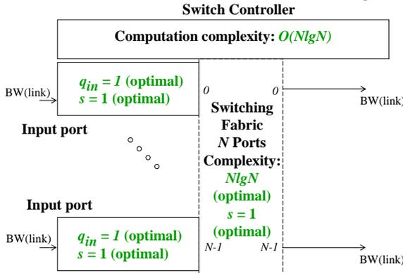
Figure 1. Optimal switch design
