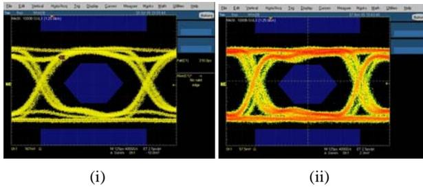
Figure 5: Eye Pattern at points: (i) 1 and (ii) 4 of Figure 4
