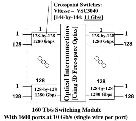
Figure 3. 160 Tb/s Switching Module (for future testbeds) based on off-the-shelf VSC3040 cross-point switches
