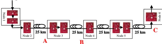
Figure 6: Metro network topology:  $4*25=100$  km fiber and 9 stages of cross-connects (or six TDS nodes)
