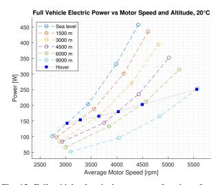
Fig. 13: Full vehicle electrical power as a function of motor speed for all the altitudes - 20 °C.
