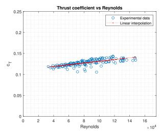
Fig. 9: Propeller thrust coefficient and Reynolds number for all the temperature and pressure.
