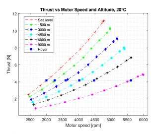
Fig. 5: Isolated rotor, Thrust - Motor Speed curve as a function of the altitude.
