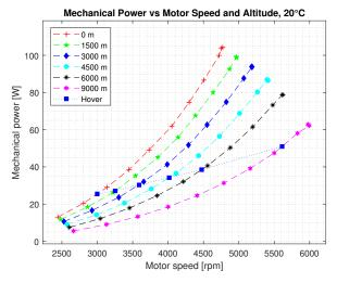
Fig. 6: Isolated rotor, Mechanical Power - Motor Speed curve as a function of the altitude.
