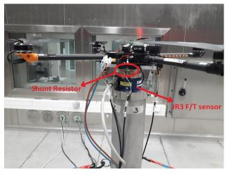
Fig. 3: Experimental setup for quad-rotor performance measurements.
