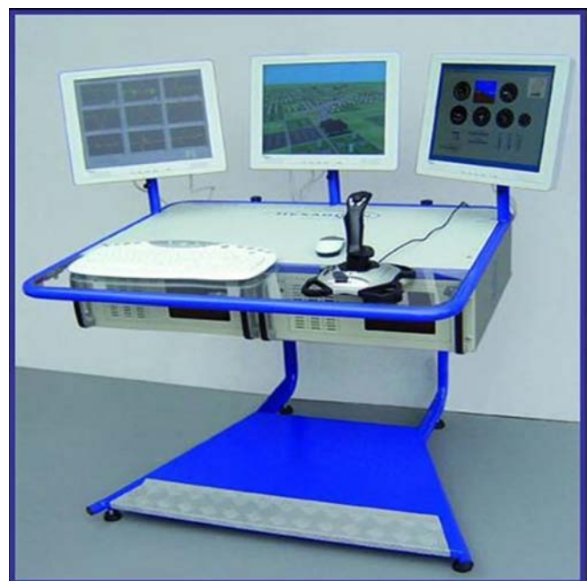
Figure 2 The HEXAGON Flight Simulator hardware
