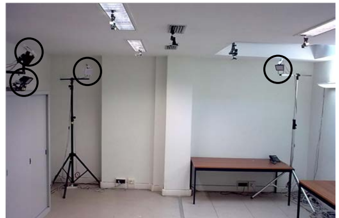
Fig. 4: MScMS-II prototype. Sensor network layout: black circles highlight the spatial position of the network device.
