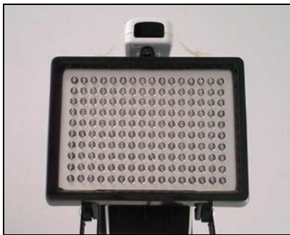
Fig. 2: MScMS-II prototype. Detail of network device: each camera is coupled with a LED array.
