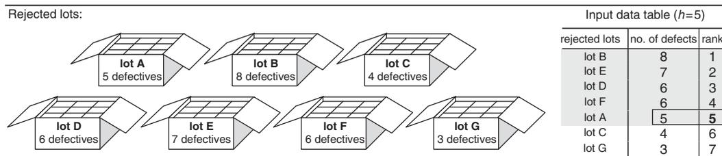
Figure 7. Use of the  $h$ -index to evaluate the Quality of supplied lots, based on the number of defective elements in each rejected lot
