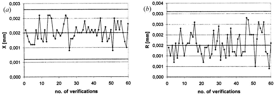
Fig. 6. (a)  $\bar{X}$  and (b)  $R$  charts of the reproducibility tests for the external witness-part during a measurement process of several successive parts on a production line. The process is in control. Control chart limits are determined on the basis of the first 20 samples. Three tests have been carried out for each measurement cycle.
