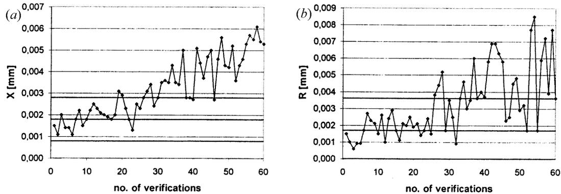
**Fig. 5.** (a)  $\bar{X}$  and (b)  $R$  charts of the reproducibility tests for the workpiece subject to a progressive increase in room temperature, after the alignment of the reference system to the measured part (see Fig. 1). The process is out of control. Control charts are determined on the basis of the first 20 samples. Three tests have been carried out for each measurement.
