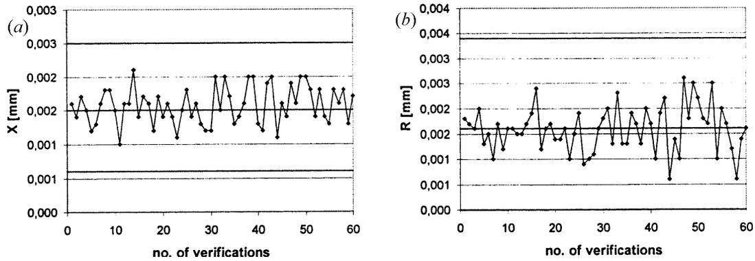
**Fig. 3.** (a)  $\bar{X}$  and (b)  $R$  charts of the reproducibility tests for the workpiece after the alignment of the reference system to the measured part (see Fig. 1). The figure shows the natural variability of the process without assignable disturbance causes. The process is in control. Control charts limits are determined on the basis of the first 20 samples. Three tests have been carried out for each measurement cycle.
