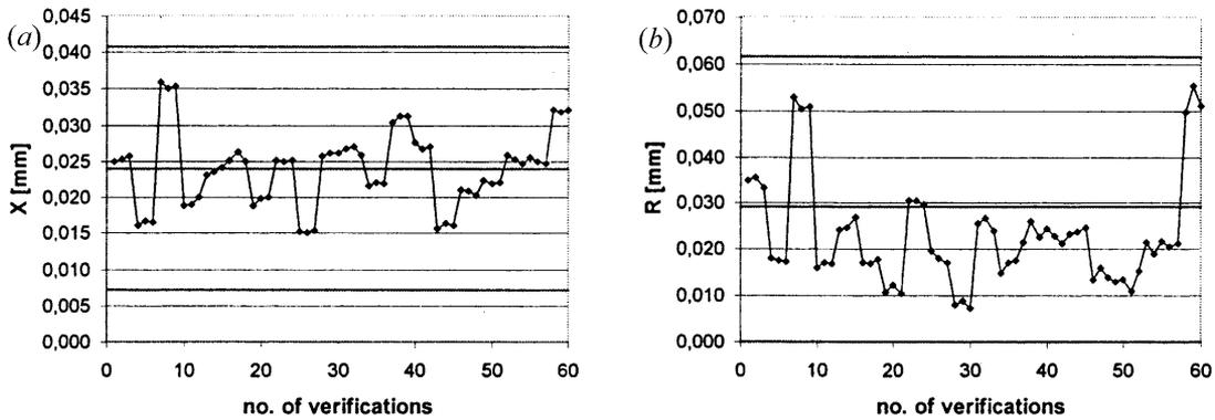
Fig. 7. (a)  $\bar{X}$  and (b)  $R$  charts of the reproducibility tests for the workpiece during a measurement process of several successive parts on a production line. The observed discontinuities reveal the effects of the positioning of a new part. The process is in control. Control chart limits are determined on the basis of the first 20 samples. Three tests have been carried out for each measurement cycle.
