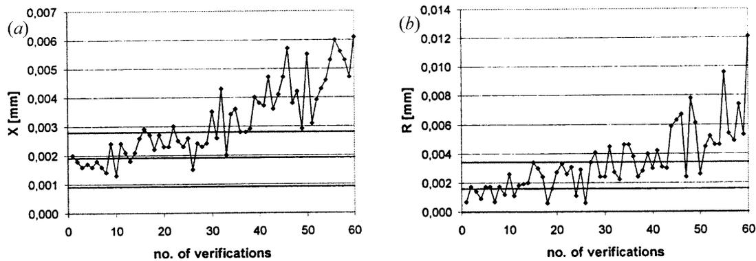
**Fig. 4.** (a)  $\bar{X}$  and (b)  $R$  charts of the reproducibility tests for the witness-part subject to a progressive increase in room temperature. The process is out of control. Control chart limits are determined on the basis of the first 20 samples. Three tests have been carried out for each measurement cycle.
