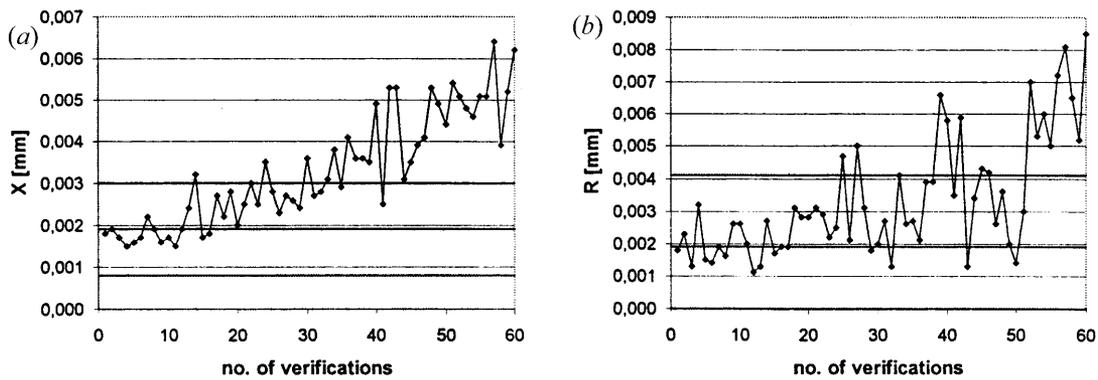
Fig. 8. (a)  $\bar{X}$  and (b)  $R$  charts of the reproducibility tests for the witness-part during a measurement process of several successive parts on a production line, subject to a progressive increase in room temperature. The process is out of control. Control chart limits are determined on the basis of the first 20 sample. Three tests have been carried out for each measurement cycle.
