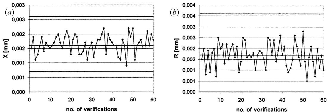
Fig. 2. (a)  $\bar{X}$  and (b)  $R$  charts of the reproducibility tests for the external witness-part. The figure shows the natural variability of the process without assignable disturbance causes. The process is in control. Control chart limits are determined on the basis of the first 20 samples. Three tests have been carried out for each measurement cycle.
