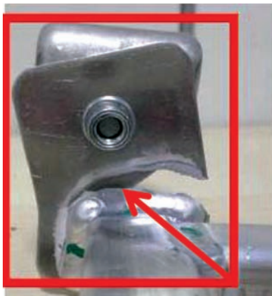
Figure 7 – Damage in a car fender
