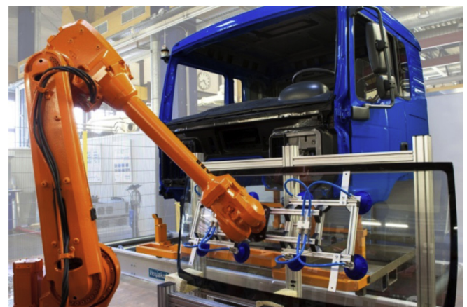
Fig. 5. Metrology based windshield assembly in motion. Source: WZL RWTH Aachen University.
