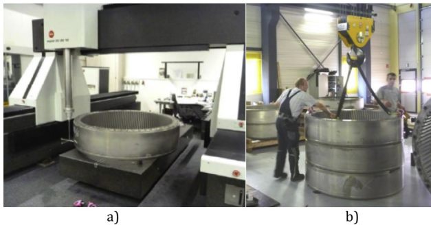
Fig. 12. Internal WES ring gear: (a) measurement using large CMM. (b) Storage, tempering and clamping of internal WES gears within a large air conditioned measuring room.
