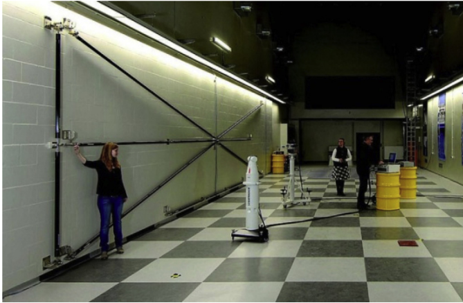
Fig. 7. PTB's new reference wall for testing and calibrating mobile 3D measuring systems for large measuring ranges (up to 10 m).
