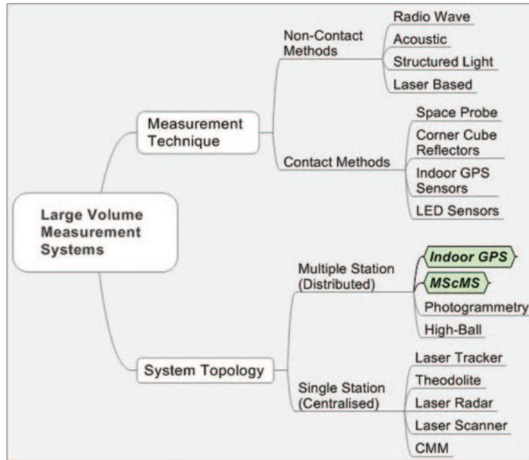
Fig. 1 Classification of large-volume measuring systems
