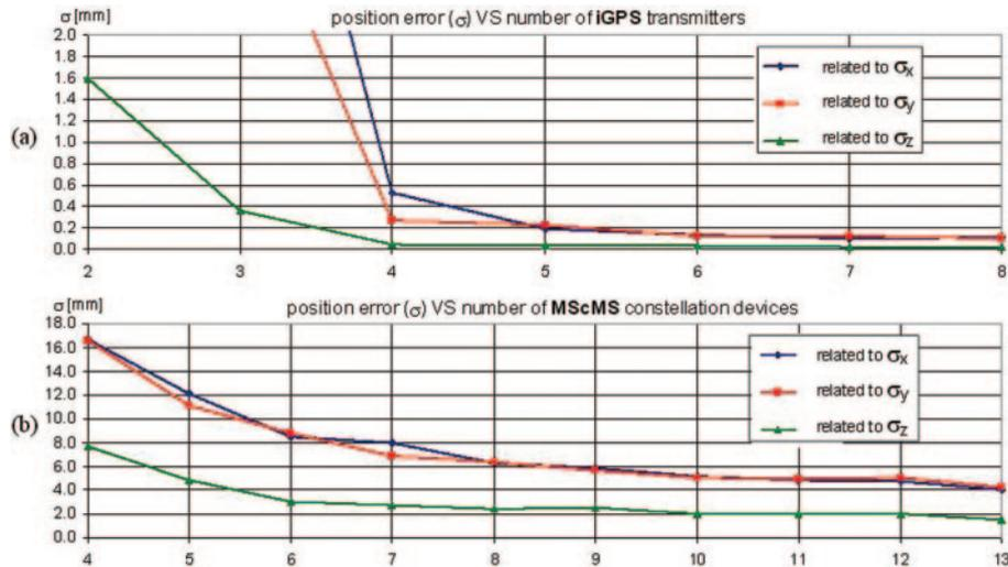
Fig. 4 Influence of the number of transmitters on the position error for the iGPS and the MScMS
