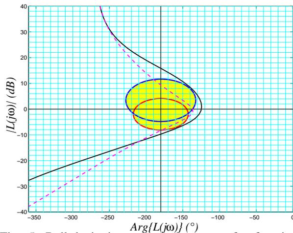
Fig. 5. Ball levitation system loop transfer function plot on the ENC:  $C_{ENC}$  (black-solid) and  $C_{mrg}$  (magenta-dashed).
