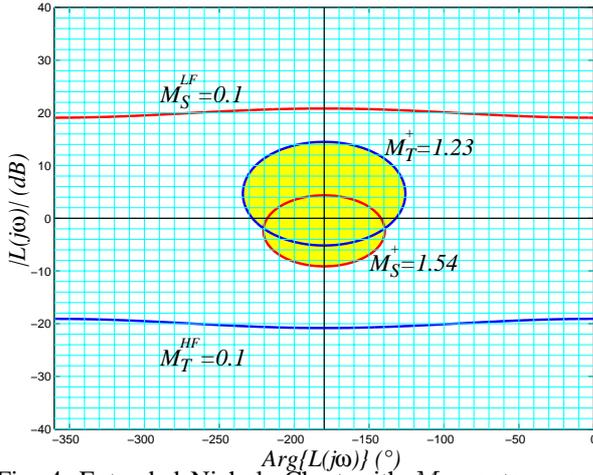
Fig. 4. Extended Nichols Chart with  $M_T$ -contours and  $M_S$ -contours.
