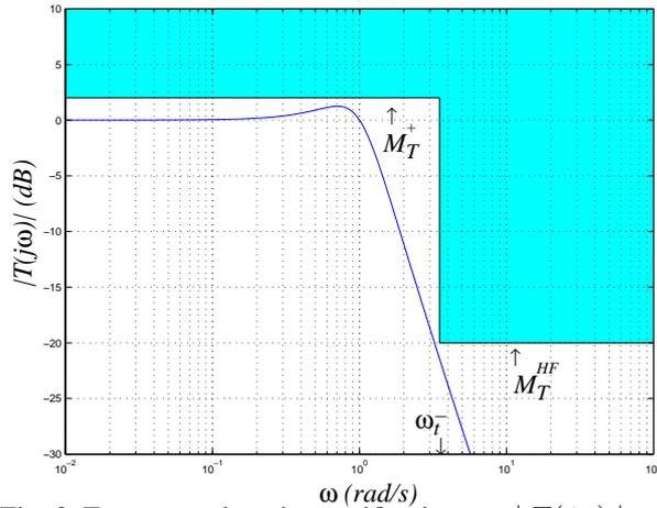
Fig. 3. Frequency domain specifications on  $|T(j\omega)|$ .
