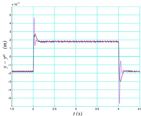
Fig. 7. Ball levitation system experimental square wave response with:  $C_{ENC}$  (black-thick) and  $C_{mrg}$  (magenta-thin).
