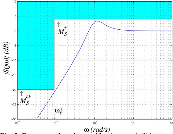
Fig. 2. Frequency domain specifications on  $|S(j\omega)|$ .
