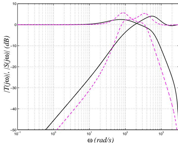
Fig. 6. Ball levitation system frequency response with:  $C_{ENC}$  (black-solid) and  $C_{mrg}$  (magenta-dashed).
