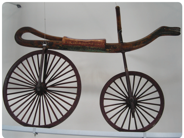
FIGURE 1 A wooden draisine with a dragon or reptile head, displayed at Deutsches Museum Verkehrszentrum, Munich, Germany. This vehicle, patented in 1817 in Germany, is the earliest known two-wheeled vehicle resembling a bicycle. The front wheel is steerable, but rotary cranks and pedals are not present, and thus a person had to push his or her feet against the ground to ride the draisine .
