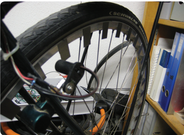
FIGURE 7 Detail of the instrumented bicycle. The encoder on the rear wheel uses a Hall effect sensor and 36 ferrous metal plates. Calculation of the speed based on the sensor pulses is performed by the AC 800PEC processing platform.
