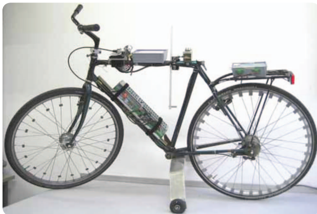
FIGURE 2 Prototype of the instrumented bicycle built at ABB Corporate Research, Baden, Switzerland, in collaboration with the Dipartimento di Automatica e Informatica of Politecnico di Torino, Italy. This prototype is based on a commercial city bicycle, from which brakes, chain, crankset, and pedals are removed. The vehicle is equipped with an encoder on the rear wheel, a rate gyro, and a potentiometer measuring the bicycle speed, roll velocity, and steering angle, respectively. Furthermore, a torque-driven servomotor provides a torque on the steering axis, while a general purpose ABB AC 800PEC includes a computational unit, a data acquisition unit, and a communication unit.
