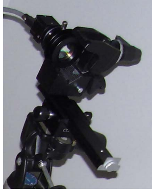
Figure 1: Contax focusing rail and the Flea2 camera fixed with a Manfrotto super clamp; the Barlow lens is not present here.
