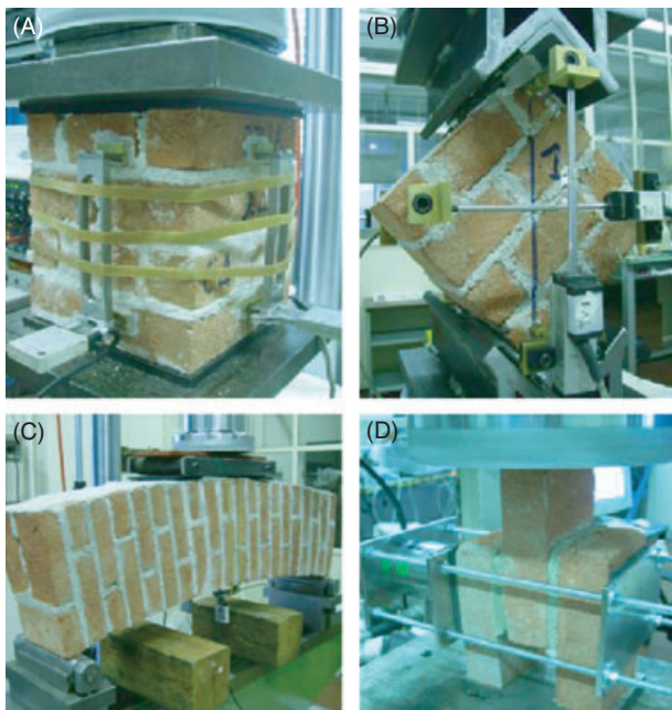
Figure 4: Laboratory tests for the mechanical characterization of the masonry: compression test (A) diagonal compression test (B) four point bending of a masonry arch (C) and shear test (D)
