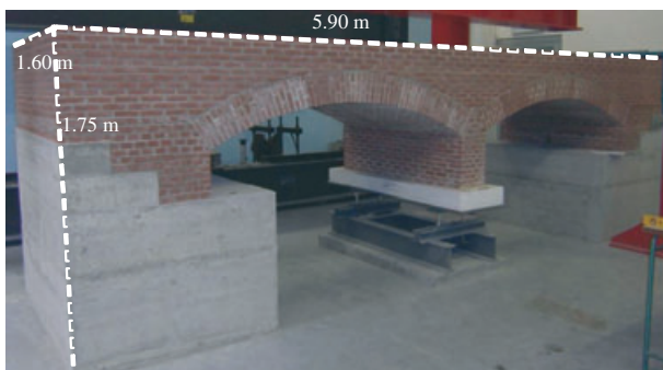
Figure 1: Model bridge realized at the Politecnico di Torino laboratories
