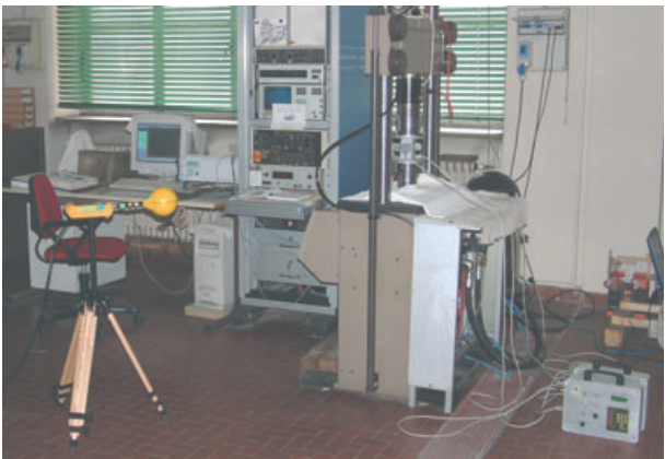
Figure 3: Photograph of the compressive test on the Green Luserna Granite specimen. The electromagnetic antenna and the acoustic emission acquisition system are shown
