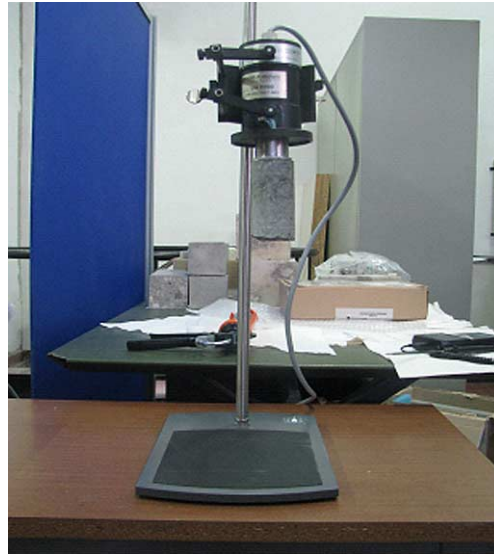
Fig. 3. The Green Luserna Granite specimen connected to the ultrasonic horn. The ultrasonic apparatus (Bandelin HD 2200) consists of a generator that converts electrical energy to 20 kHz ultrasound, and of a transducer that switches this energy into mechanical longitudinal vibration of the same frequency. (Colors are visible in the online version of the article; http://dx.doi.org/10.3233/SFC-2011-0120 .)
