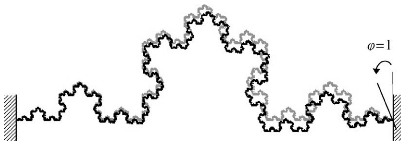
Fig. 6. Elastic deformation of a six-order von Koch beam clamped at both the ends and subjected to a unitary counter-clockwise rotation of the right end.
