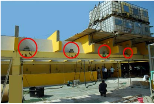
Fig. 7 Photo of the loading apparatus. Circles denote the positions of the attached ATEL® AE transducers. Transducer No. 1 is on the left
