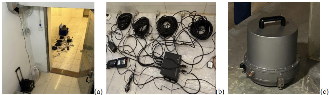
Figure 5. Setup of monitoring system. (a) Interior view of the tunnel, (b) AE acquisition device and (c) seismometer.
