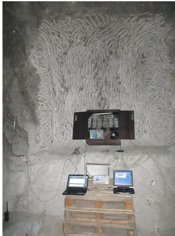
Fig. 3. The monitoring station equipped with the AE piezoelectric sensors, the telescopic antenna and oscilloscope for EME evaluation, and the NE proportional counter.
