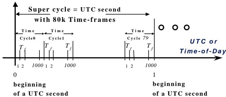
Figure 8: CTR™ with time frames  $T_f = 12.5 \mu s$
