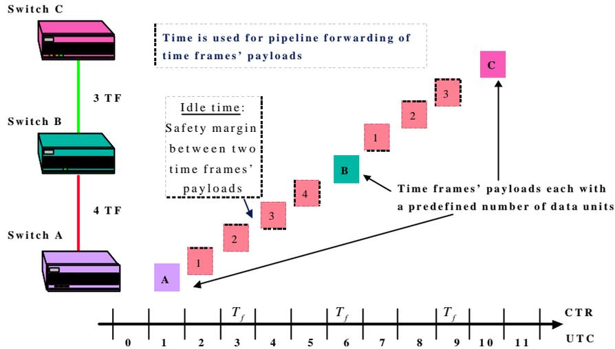
Figure 7: Pipeline Forwarding (PF™) of time frames
