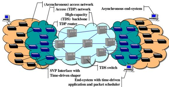
**Fig. 2. Architecture for deploying pipeline forwarding**
