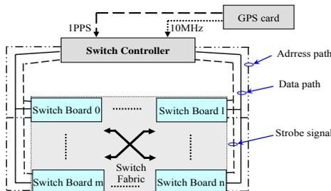
**Fig. 4. TDS switch block diagram**
