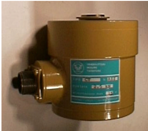
Fig. 1. Picture of the force transducer used as a transfer standard for the verification of the automatic-force-controlled Rockwell Hardness machine.
