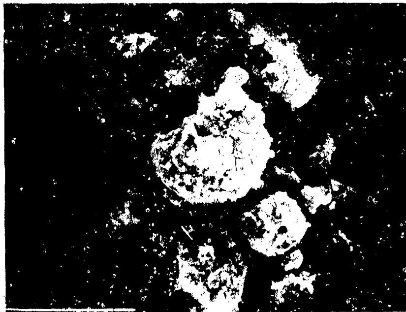
Figure 7. Demonstration of Particle Breakup as a Result of Inherent Fragility; Small Bar Represents 5 \mu\text{m}
