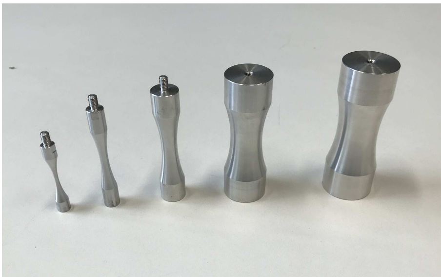
FIGURE 2 The five different tested hourglass and dog-bone specimens. [Colour figure can be viewed at wileyonlinelibrary.com ]
