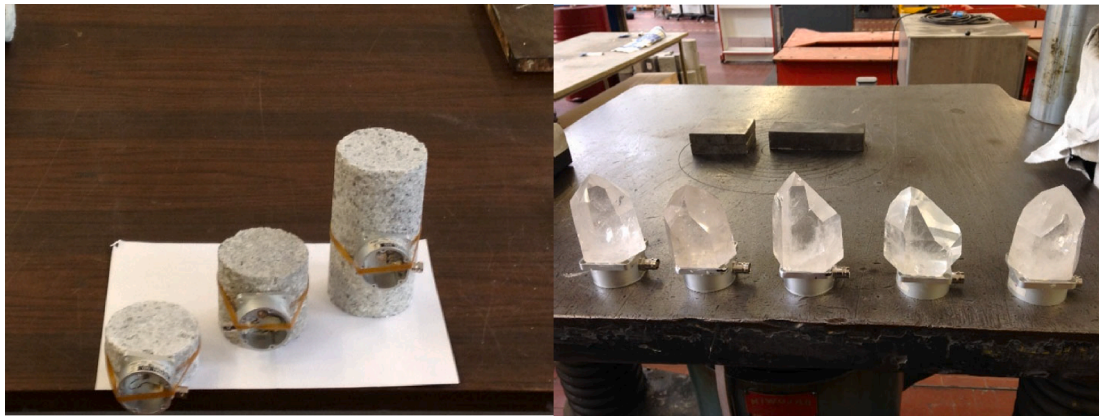
Fig. 1. Gypsum specimens varying the slenderness (left) and Quartz specimens with irregular shapes (right).
